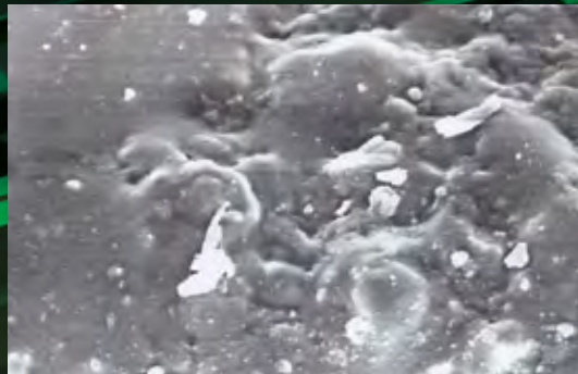
Tile reverse side: Tile Smooth pore structure on the adhesive surface of the stoneware slab with poor adhesion properties, SEM image at 500X magnification – direct view.
