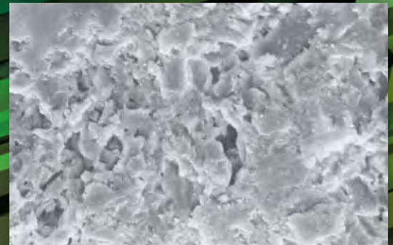
Tile reverse side: STRÖHER Keraplatte® Keraplatte® programme with very good adhesion properties, SEM image at 500X magnification – direct view.
